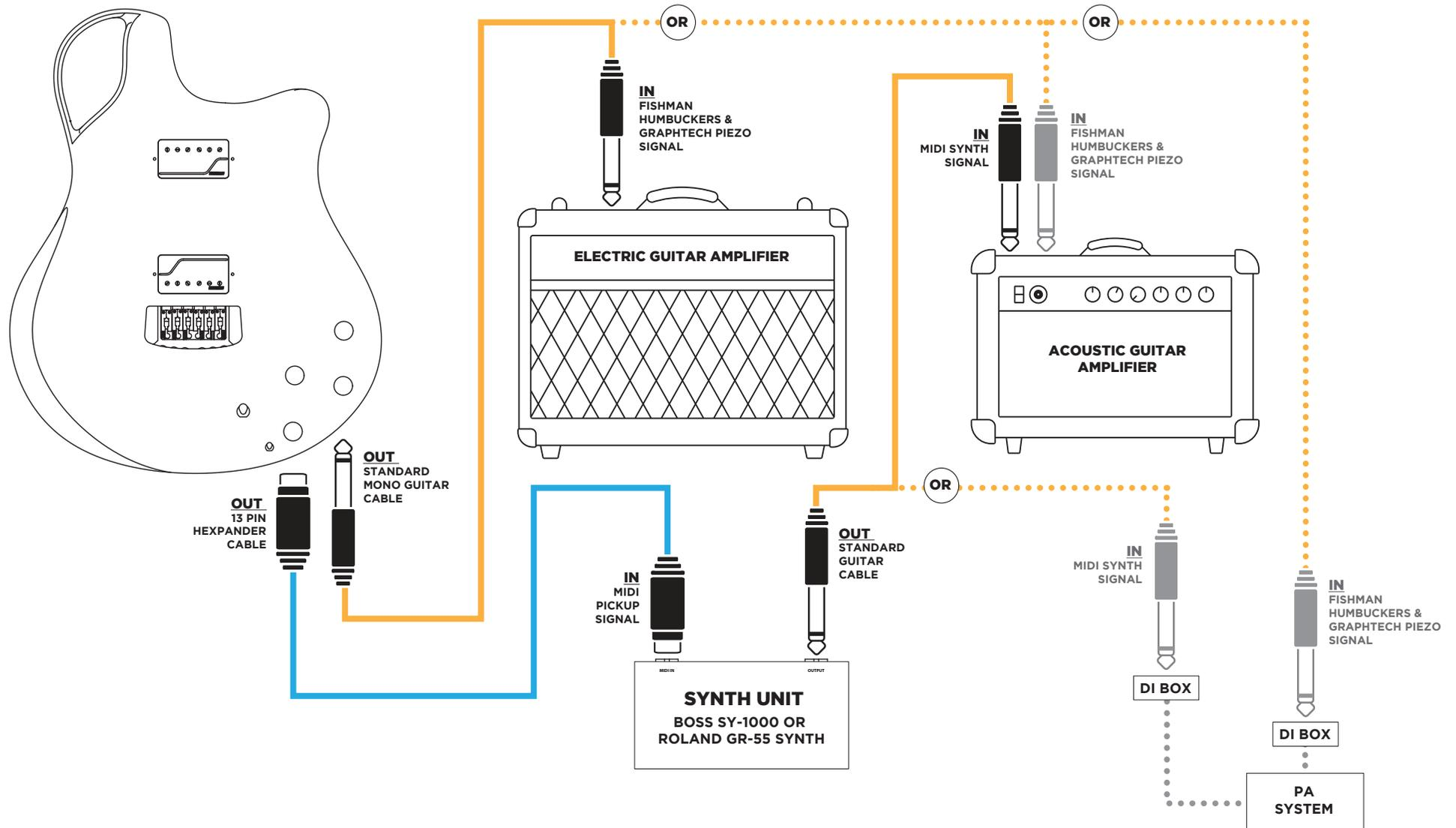
13 Pin Hexpander    Stereo to x2 Mono Guitar Cable    Standard Mono Guitar Cable
